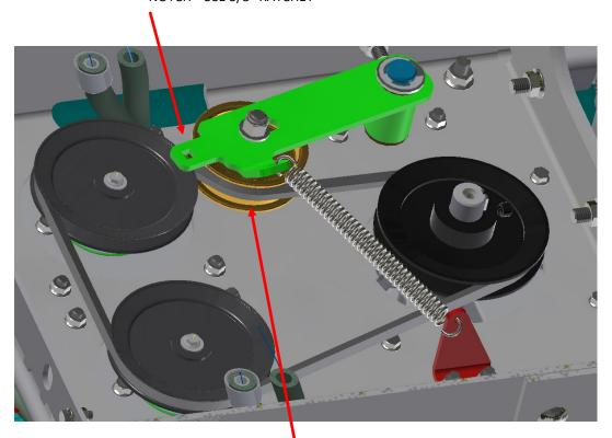
**NOTE:** Be sure the engine belt is on the proper side of the idler arm.
