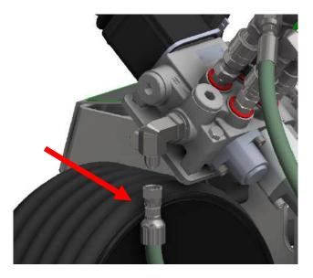
• Attach the other end of the hose to the input port of the hopper control valve. (end with 90° fitting)
