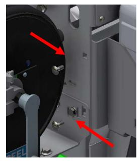
• Attach the control valve assembly to the side of the upright using (2) 3/8 X 1" carriage bolts provided with the kit and reuse the nuts that were removed.
